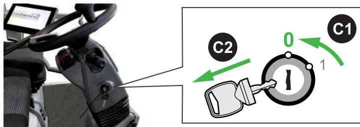
Disconnect high-voltage by switch off "ignition" (C1) of the vehicle. Remove the key (C2) and store it safely.
