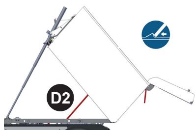
Raise to the fully raised tipping position and ensure that the safety props (D2) engage.
