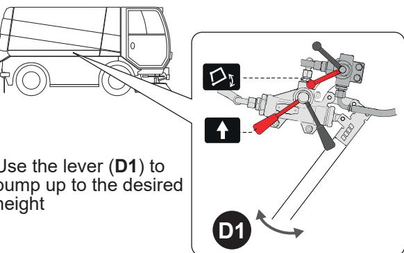
Use the lever (D1) to pump up to the desired height
