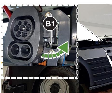
Open the right side flap on the hopper (B1). For emergency unlock, move the lever (B2) behind the plug socket to the right..
