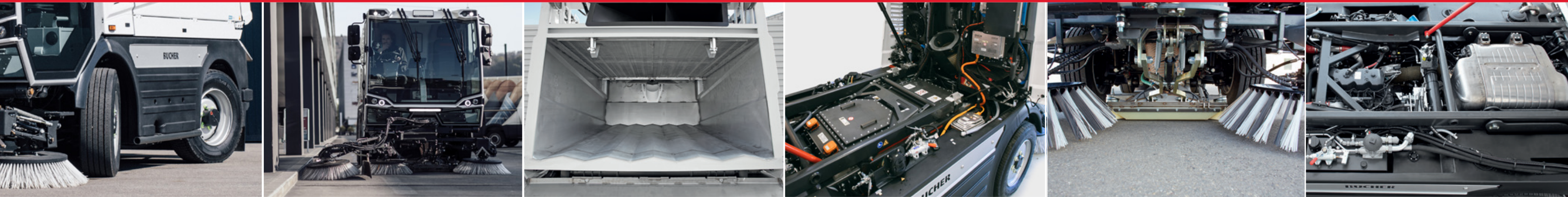
4 wheel steering 3 rd brush 5.6 m³ Hopper 137 kWh Bucher Battery Pack Wide suction intake 118 kW, Euro 6 emission diesel engine
